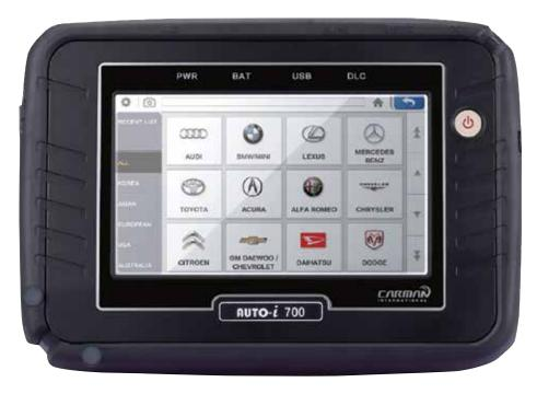
repairer simply reads and records the original PIN code that is required during the re-coding of the immobiliser after the ECU has been replaced. This feature is indispensable when new keys may require programming.
